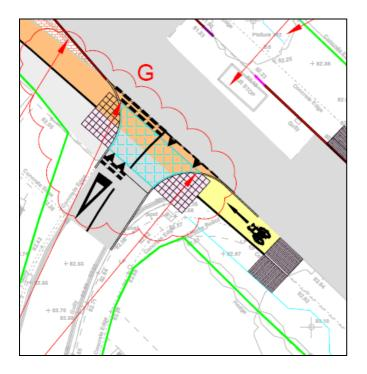
We would like to see the footway and cyclepath continuous in both level and material to reinforce the pavement, with no vehicle edge provided by the kerb-line.
