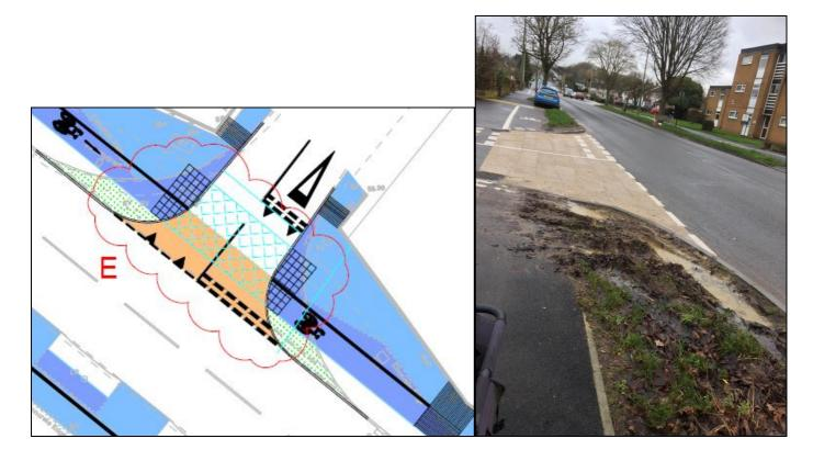
Despite the reduced radii, this junction is compromised and unacceptable without the ramp shown in the drawing as the radii are still too generous for a quiet residential road.
